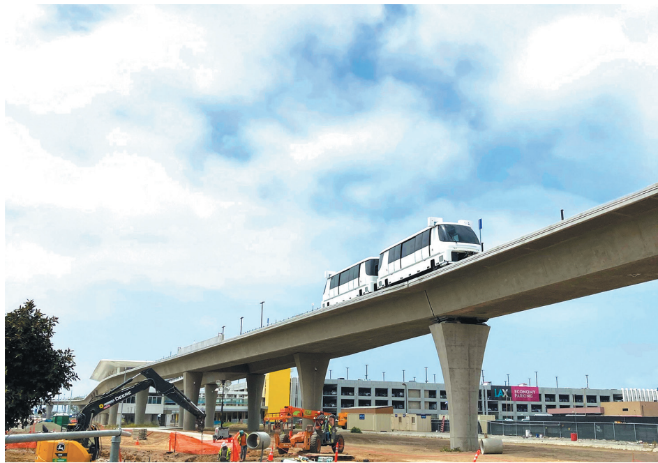
THE FIRST PAIR of APM train vehicles cross Century Boulevard on the elevated guideway. Photo courtesy of Los Angeles World Airports.
